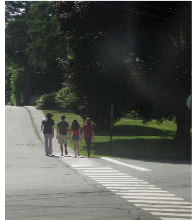
Wide curb radii lengthen the crossing distance for pedestrians and discourage motorists from slowing down to turn the corner.
